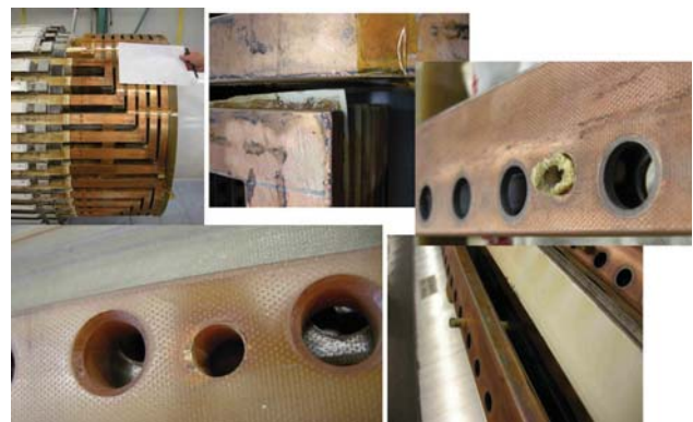
Figure 4. Power Plant Voerde Generator rotor damages.
