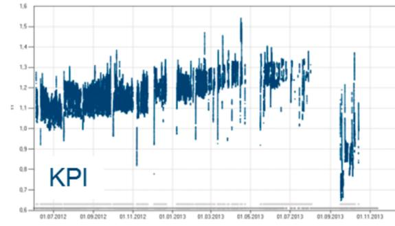
The temperature downstream of the high-pressure bypass can be used as an indicator of a leakage. When the high-pressure bypass is closed, the temperature will decrease to a plant-specific minimum value. This value will rise with an increasing leakage.
