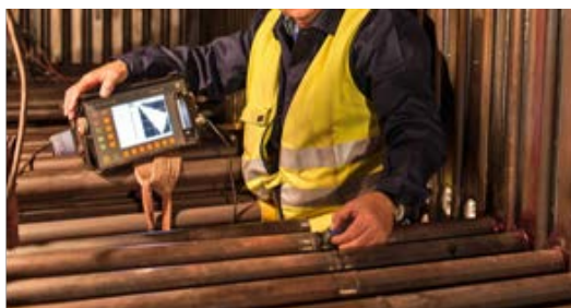
Fig. 1: Portable Phased Array Ultrasonic Flaw Detector Phasor XS™
